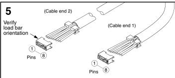
· Orient load bar with contact slots facing downward.
