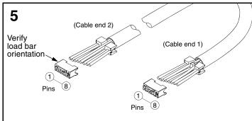
• Orient load bar with contact slots facing downward.
