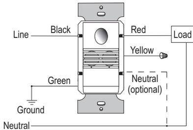
Simple optional neutral connection allows installation in any 2-wire or 3-wire application. When used in a multi-way application, all devices in that space must be wired using the same method of either with neutral or without neutral.
