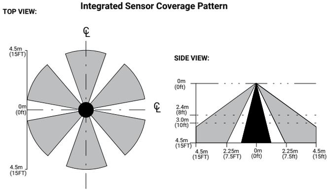
**Note:** Installation of integrated sensors within 3-ft (1m) of HVAC air vents is not recommended. The pattern shown is intended solely as a general guide and is not to scale.
