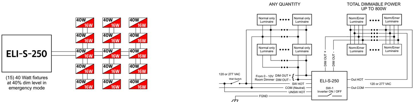
(15) 40 Watt fixtures at 40% dim level in emergency mode
