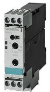
Analog monitoring relay Fill level monitoring Resistance monitoring from 2 to 200 kohm 0vershoot and undershoot 24 to 240 V AC/DC 50 to 60 Hz DC and AC 2-step or 1-step control Tripping delay 0.5 to 10 s 1 change-over contact screw terminal Successor product for 3UG3501
