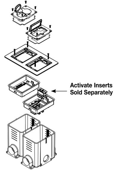
Flush installation with Ortronics® installed using 829PFLRT Cover or Activate installed using 829PFL Cover.
