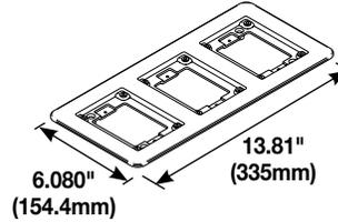
**Three-Gang Brass Combination Carpet and Tile Flange** – Accepts Ortronics® MAB6TJ TracJack and MAB3S2 Series II adapters and Wiremold CM Series inserts, sold separately.
