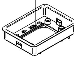
**Nonmetallic Floor Box Adjusting Ring –** Comes with fiber storage loop. Also includes brass inserts for flange connection and green ground wire for ground connection. Activate modular inserts snap directly into the adjusting ring without the need for a bezel. Also includes mounting screws to attach flange to box body. Ortronics® connectivity inserts do not snap directly into the adjusting ring. For Ortronics® inserts use the 828GFITC or 829PFLRT.
