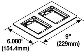
**Two-Gang Brass Combination Carpet and Tile Flange** – Accepts Ortronics® MAB6TJ TracJack and MAB3S2 Series II adapters and Wiremold CM Series inserts, sold separately.
