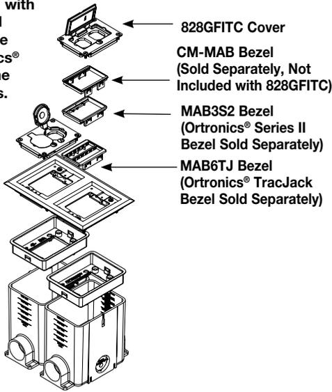
Recessed installation with Activate installed directly into the 880MPA Adjusting Ring. Ortronics® inserts cannot be inserted directly into 880MPA, see below for Ortronics® solution.
