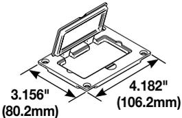
**Brass GFI Cover Plate** – May be used with Activate and Ortronics® Connectivity Systems in conjunction with 817B, 827B, and 837B Flanges.
